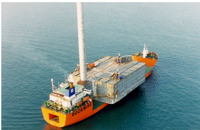
Dry-tow of storage tank
